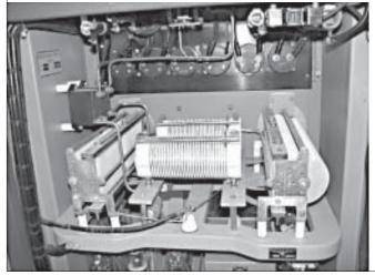
capacitors, mica transmitting capacitors (2000 pf, 6kV), ball handle toggle switches, ceramic coil form 2.5" OD, silver plated #16 AWG wire, Collins (or similar) tuning coil cans, correct tube shields, RF ammeter, 2.5 to 3 amps.
