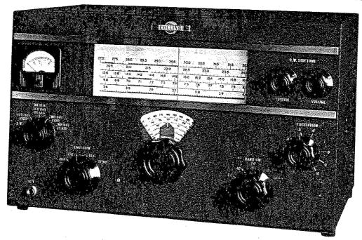
The 310A-3 exciter unit for the 30K-1 has a Collins 70E-8A PTO, and an r-f output of 10 watts. All circuits are ganged together and controlled by a single tuning knob. The slide rule dial gives a rough indication of operating frequency, while the vernier dial provides a direct reading in kilocycles. Both accuracy and stability are very high. The PTO operates in the 160 meter band. The output tube in the exciter is an 807 which is used as a doubler on all bands except 80 meters.
