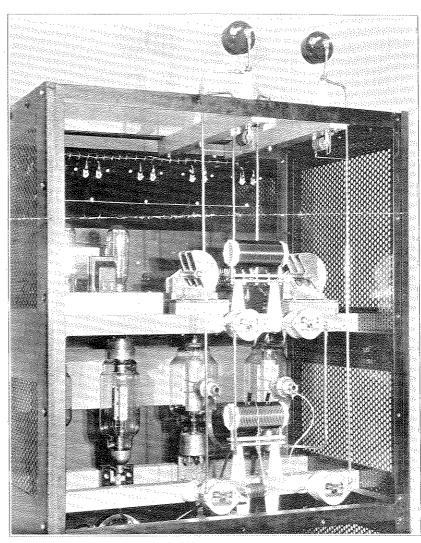
Two Federal F-100A tubes are used in pushpull in the class C stage. The plate input to these tubes is normally 1.5 kw. (0.5 ampere at 3,000 volts.) The 750 watts of audio power required to modulate this input is obtained from the two 849 class B modulators. The Federal tubes give excellent account of themselves and operate efficiently in this transmitter on frequencies up to 30 mc. The tubes have plain tungsten filaments which draw 50 amperes at 11 volts.
