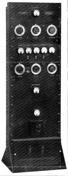
unit, 1200C power supply. These units are assembled in the 150B rack with appropriate meters and panels and are interconnected by means of a special interunit cable. Electrical design and mechanical construction are consistent with usual Collins practice.
