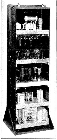
fidelity. The 7B amplifier is the only external speech equipment required exclusive of microphones. Provision is made in the 150B transmitter to receive the output of the 7B amplifier over a short shielded line.
