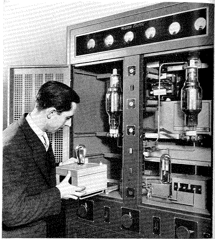
Fig. 5—Placing crystal oscillator unit in the transmitter.
